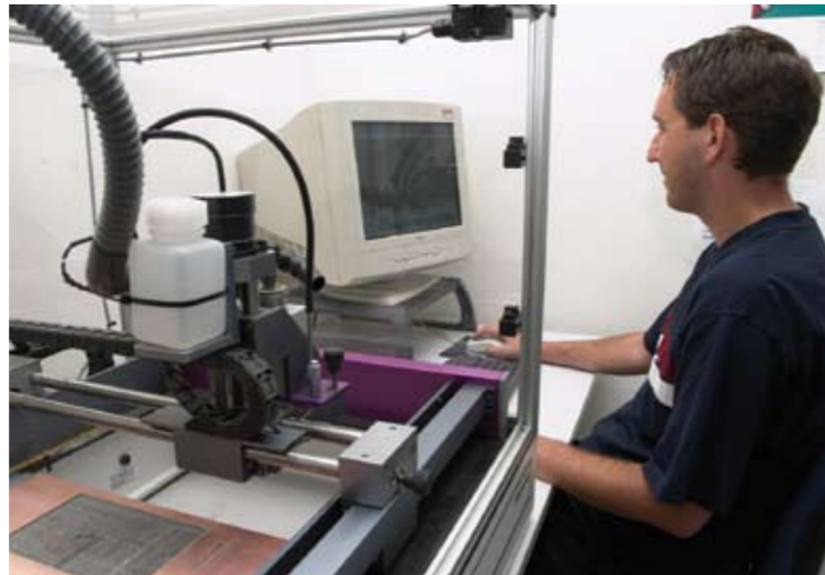
Figure 2: The laboratory milling machine gets a prototype PCB ready in minutes.
