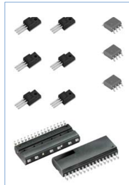
Figure 5: Needed devices for a dishwasher rinse pump application Top, discrete solution; Bottom SMD.
