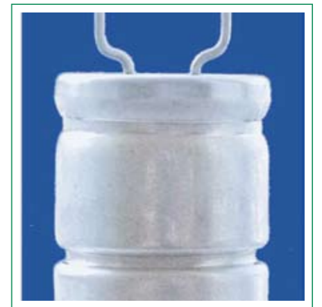
Figure 3: Snap-in electrolytic capacitor with additional centre corrugation. The snap-in models are complemented by the large-size design in which wires instead of snap-in clamps are welded to the feed-throughs. This version is also available with customer-specific bent wires and without insulation.
